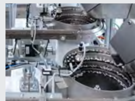
e.g.: Feed systems for correctly positioned component provisioning
