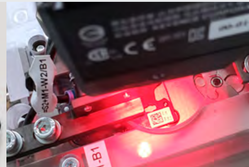
An integrated barcode scanner ensures a verifiable production process.
